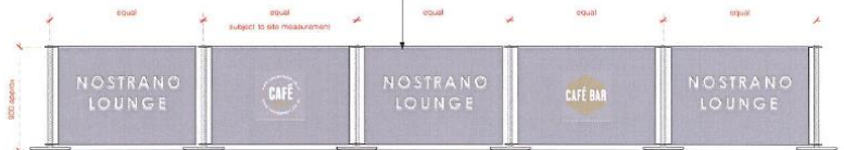
Typical Elevation of Cafe Barriers @ 1:20
