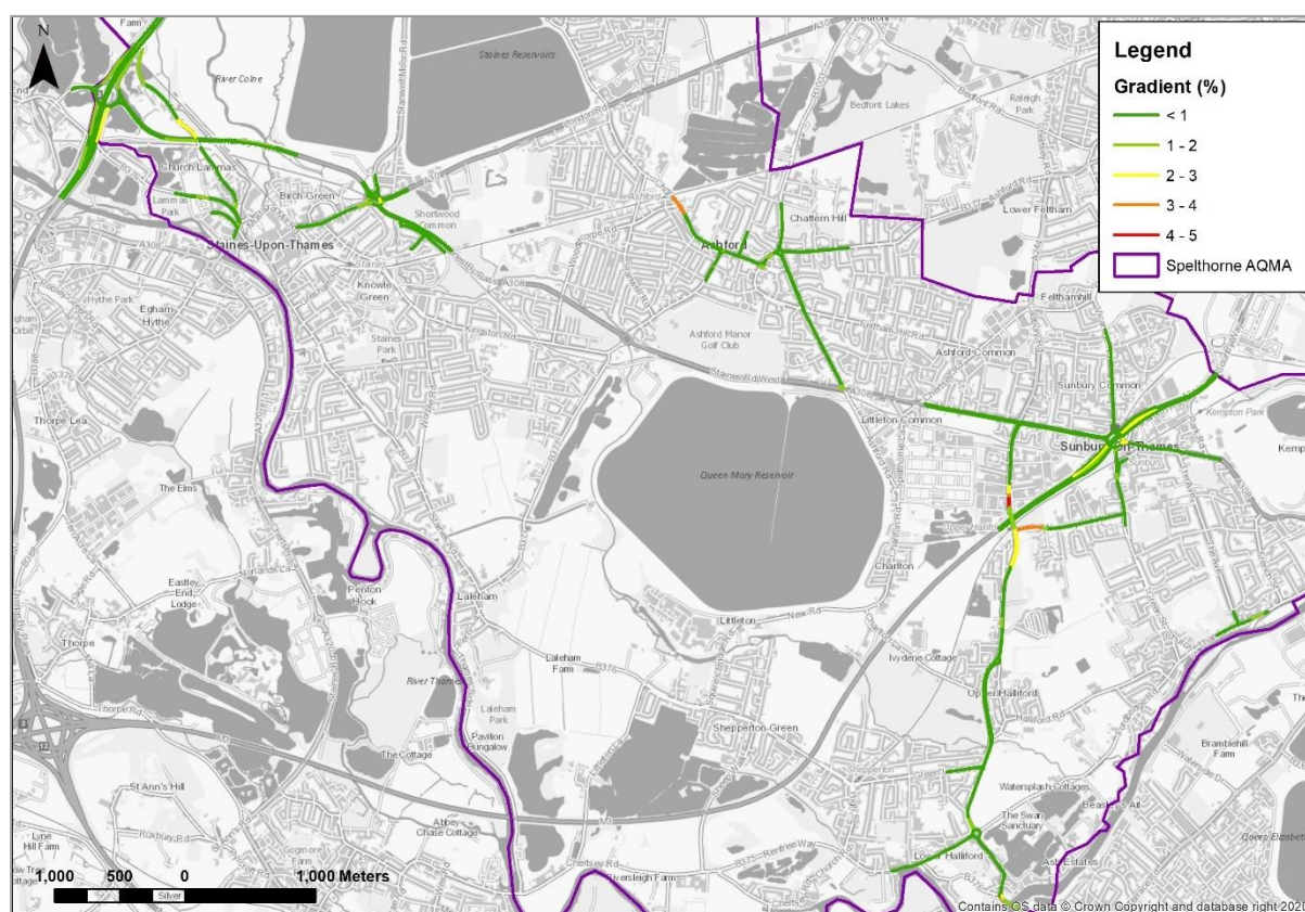
Figure 2.9: Road link gradients calculated using GIS analysis of LIDAR DSM datasets
