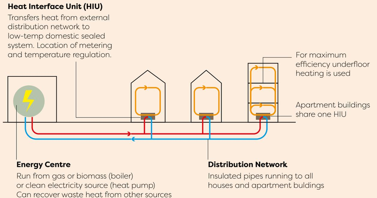
FIGURE 8: HOW HEAT NETWORKS WORK
